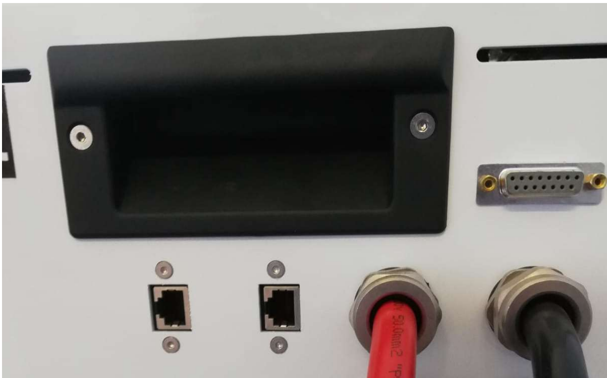
Figure 4.2 Picture Showing 2 x RJ45 Sockets for CAN Bus (DB15 Plug shown here for Analogue and Relay Control is not available in new models)
