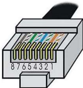
Fig 4.1 Pin Configuration for standard RJ45 plug
